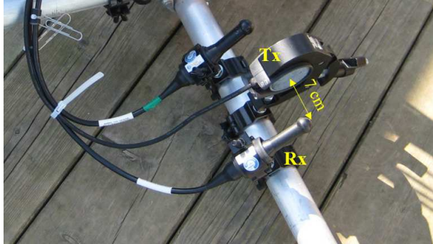
Figure 8: Transducer (Tx) and hydrophone (Rx) used in the lake experiment. Note that the other hydrophone with the green label is not used in this experiment.
