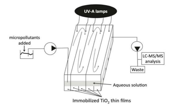
Figure 9 Continuous flow reactor for photocatalytic degradation of micropollutants (Carbonaro et al., 2013) reprinted with permission from Elsevier.
