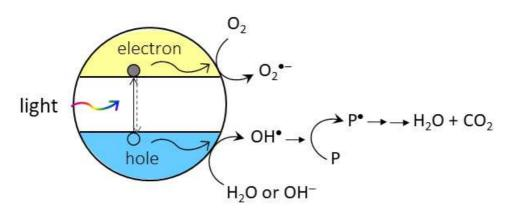
As the first step in photocatalysis, a photon of light with the energy higher than the bandgap energy of the photocatalyst material is absorbed by the photocatalyst particle. This is the photoexcitation
