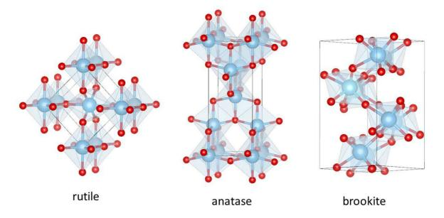
Figure 6 Bulk structure of TiO<sub>2</sub> rutile, anatase and brookite
