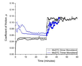
Fig. 16 Durability of the monoblend MoDTC dimer (black) and MoDTC trimer (blue) tribofilms (Color figure online)
