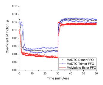
Fig. 17 Durability of the fully formulated MoDTC dimer (black), MoDTC trimer (blue), and molybdate ester (red) tribofilms (Color figure online)
