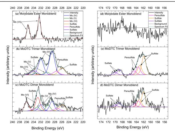
Fig. 11 Mo 3d (left) and S 2p (right) regions of molybdate ester (top) MoDTC trimer (center) and MoDTC dimer (bottom) monoblend oil tribofilms
