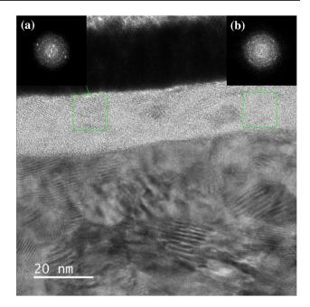
Fig. 13 MoDTC Trimer tribofilm crystallinity regions with inset FFTs of a crystalline and b amorphous regions
