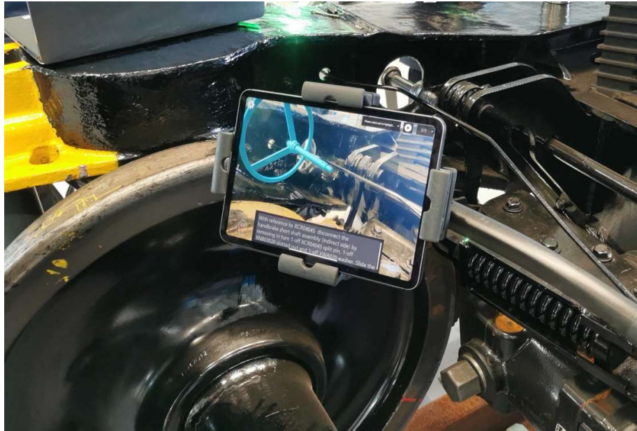
Figure 9. Example AR overlay for identifying service and maintenance items on a train chassis.
