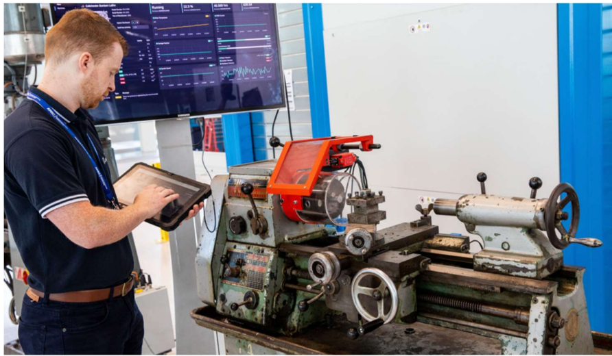
Figure 4. Colchester Bantam lathe with a low-cost Industry 4.0 solution (Lockwood et al., 2018).
