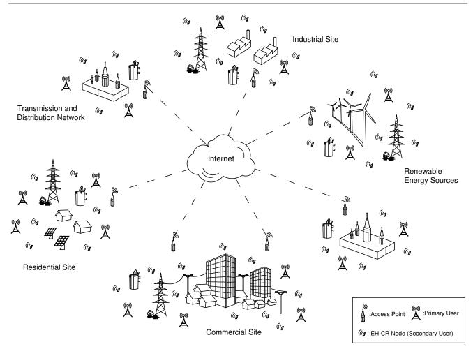
Fig. 1 IoT-enabled SG Architecture.
