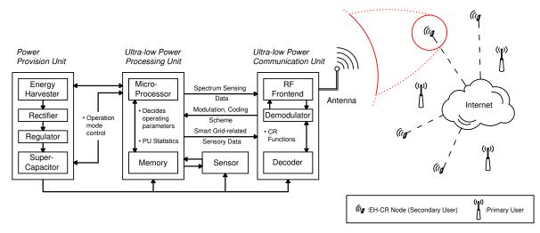
Fig. 2 Node Architecture of EH-CRs.
