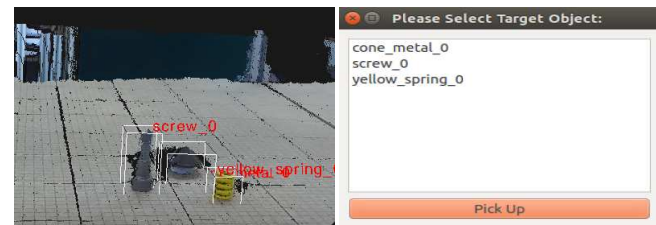
(b) Visualization of detection result (c) The pick up list of detected object instances
