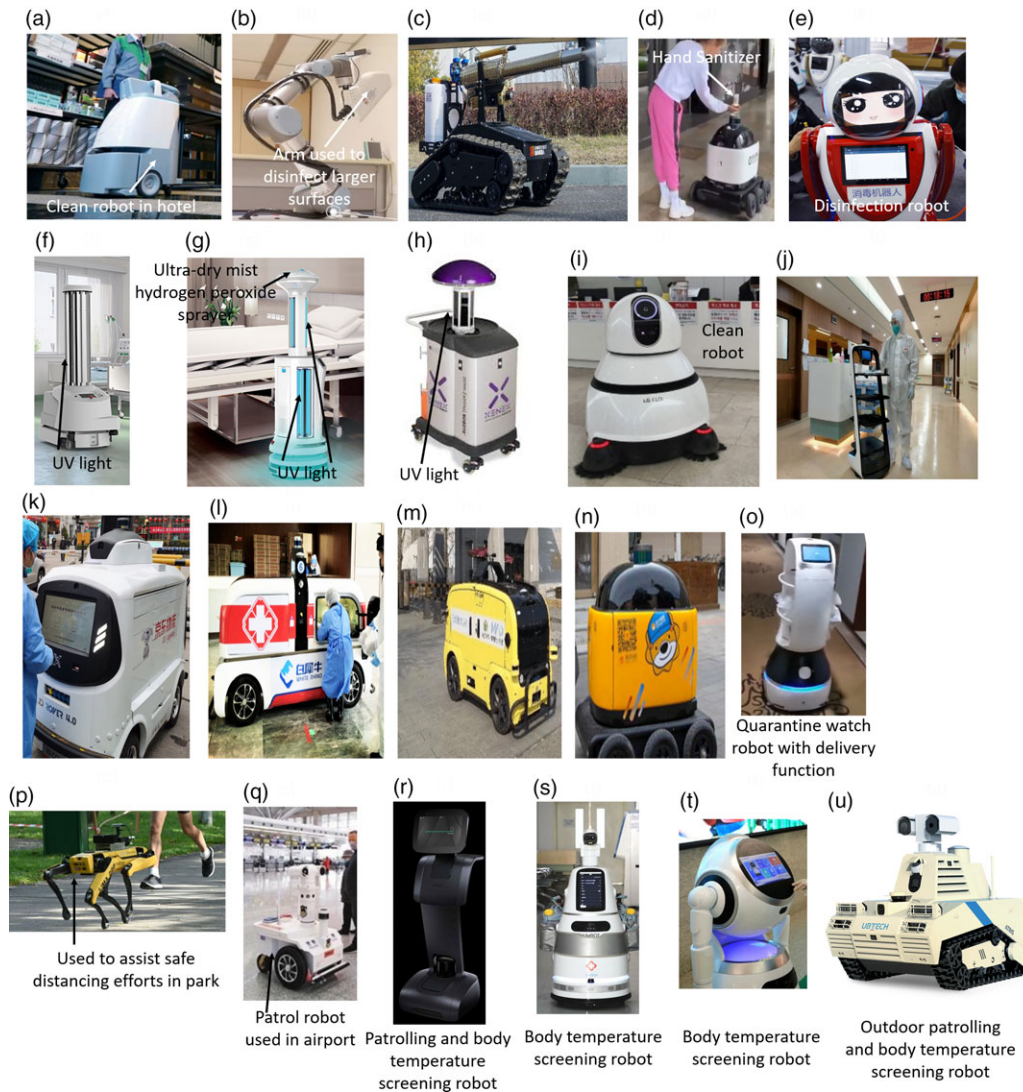
Figure 2. (a) Cleaning Robot from SoftBank Robotics. 8 (b) XDBot by Nanyang Technological University. 9 (c) Tank-style, remote-controlled disinfecting robot. 10 (d) Portable hand sanitizer robot from Zhen Robotics Corp. 11 (e) Aerosol Disinfection Robot from Shanghai TMI Rob Technology. 12 (f) UV-C light Disinfection Robot by UVD Robots. 13 (g) Intelligent Disinfection Robot by TMI Rob. 14 (h) UV light robot by Xenex Disinfection Services. 15 (i) Autonomous Cleaning Robot by Seoul National University Hospital. 16 (j) Pudu Technology's autonomous service delivery robot. 18 (k) JD Logistics' large self-driving delivery vehicle. 19 (l) White Rhino Auto Company's large self-driving delivery vehicle. 20 (m) Meituan's large self-driving delivery vehicle. 21 (n) ZhenRobotics' RoboPony. 22 (o) Quarantine watch robot. 23 (p) Boston Dynamics' Spot being used in Bishan-Ang Mo Kio Park, Singapore. 24 (q) Smart patrol robot being used in Guiyang Airport, China. 25 (r) Temi robots, 26 (s) AIMBOT, and (t) Cruz robots from UBTECH. 28 (u) Atris outdoor screening and patrolling robot from UBTECH. 30
