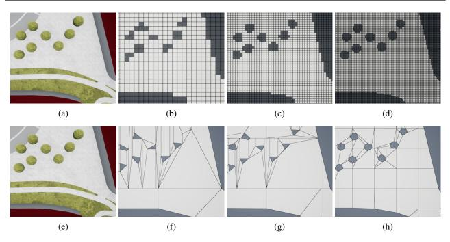
Figure 26: Grid and navmesh representation of the environment. Top row shows three grids with different resolutions: (a) original environment, (b) 128x128, (c) 256x256 and (d) 512x512. Bottom row shows three navmeshes with different voxel size: (e) original environment, (f) 0.5, (g) 0.25 and (h) 0.1.
