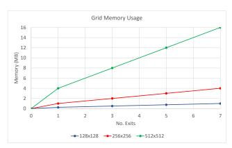
Figure 27: Memory used in megabytes (MB) by three grid sizes and multiple exits: 128x128 (blue), 256x256 (red) and 512x512 (green).
