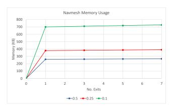
Figure 28: Memory used in kilobytes (kB) by three navmeshes with different voxel size and multiple exits: 0.5 (blue), 0.25 (red) and 0.1 (green).
