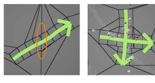
Figure 7: Polygons misaligned when crossing tile boundaries.
