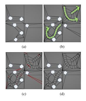
Figure 9: (a) Four tiles of the navmesh. (b) The same four tiles with three flow lines sketched by the user. (c) Recast's polygon merge algorithm creates 148 polygons. Edges that are eliminated by our improved algorithm are highlighted in red. (d) The 130 polygons resulting from the improved algorithm.
