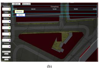
Figure 11: (a) Simple scenario with one entrance (yellow), one barrier and one exit (red). (b) Timeline simulating two events. The emission rate of the entrance is increased, and the barrier appears shortly after that.
