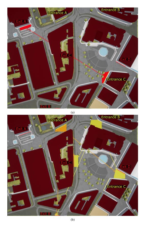
Figure 19: Crowd marshalling scenario. (a) The crowd to be marshalled spawns from Entrance C and moves towards Exit A. (b) Pedestrians walking around the city move from Entrances A and B to Exits B, C and D.
