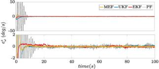
**FIGURE 1** Angular velocity estimation error (process noise-case 1). *X*–*Y*–*Z* component (from top to bottom)
