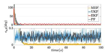
**FIGURE 8** Attitude estimation error  $e_{q,R}(t)$  (deterministic model error -case 2)
