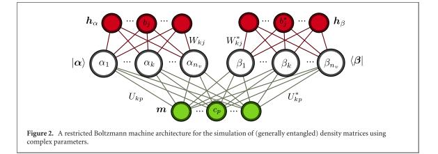
The inherent advantage offered by the RBM architecture for generative modelling is that there are no *intra*-layer connections (i.e. there are no connections between adjacent visible units or hidden units). This allows for an ansatz that is independent from the activations of the hidden state space. Thus, one can define a positive NNS wavefunction as [12]
