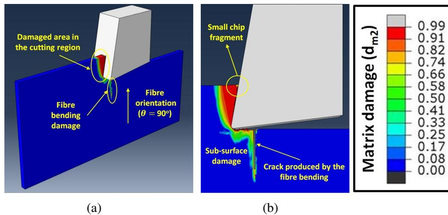
**Fig. 10.** Representation of the FE model simulated with a fibre orientation of 90°: (a) 3D perspective view (b) Front view
