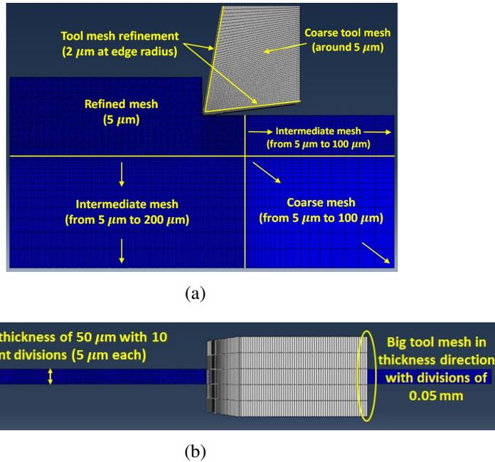
**Fig. 2.** Representation of meshed areas of the model: (a) Laminate and tool mesh distribution (b) Mesh distribution in the thickness
