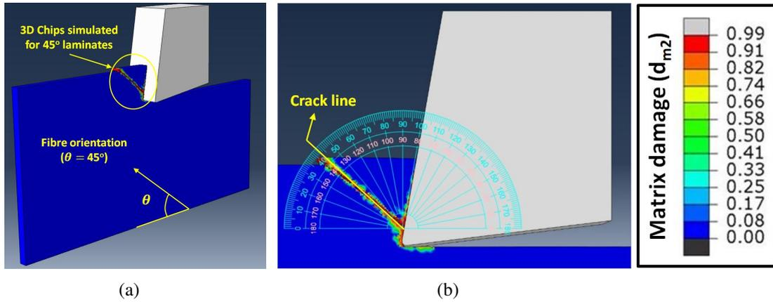
**Fig. 8.** Representation of the FE model simulated with a fibre orientation of 45°: (a) 3D perspective view (b) Front view
