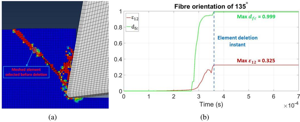
**Fig. 14.** Representation of a representative meshed element deleted to simulate the chip of laminates with a fibre orientation of 135°: (a) Meshed element selected before deletion (b) Evolution of  $d_{fc}$  and  $\varepsilon_{12}$  during the simulation time.
