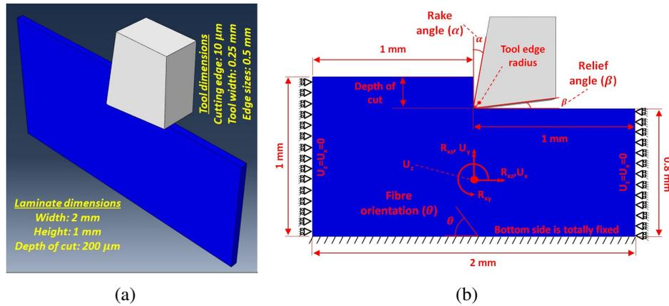
**Fig. 1.** Representation of the FE model simulated: (a) 3D perspective view (b) Boundary conditions and relevant cutting parameters modelled
