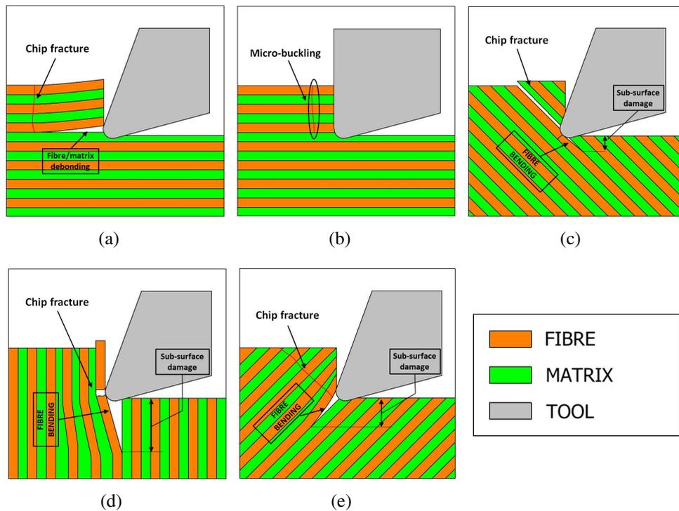
**Fig. 3.** Representation of the different chip fracture scenarios studied in this research: (a) Fibre orientation of  $0^\circ$ , (b) Fibre orientation of  $0^\circ$  with a rake angle of  $0^\circ$ , (c) Fibre orientation of  $0^\circ$  with a rake angle of  $0^\circ$ , (d) Fibre orientation of  $90^\circ$  and (e) Negative fibre orientations or superior to  $90^\circ$
