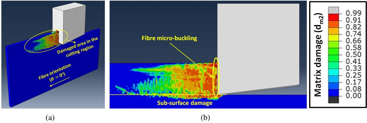
**Fig. 6.** Representation of the FE model simulated with a fibre orientation of  $0^\circ$  and a rake angle of  $0^\circ$ : (a) 3D perspective view (b) Front view
