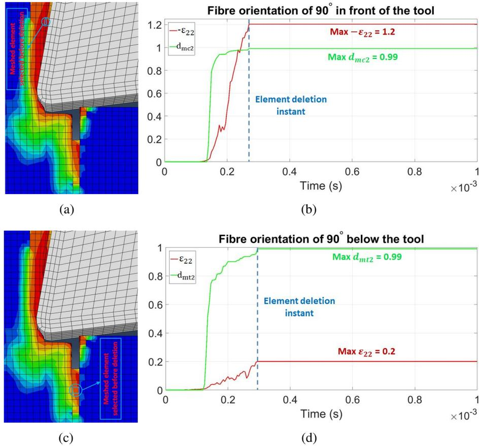
**Fig. 11.** Representation of a representative meshed element deleted to simulate the chip of laminates with a fibre orientation of 90°: (a) Meshed element selected in front of the cutting tool before deletion, (b) Evolution of  $d_{mc2}$  and  $\varepsilon_{22}$  during the simulation time, (c) Meshed element selected below of the cutting tool before deletion, (d) Evolution of  $d_{mt2}$  and  $\varepsilon_{22}$  during the simulation time.
