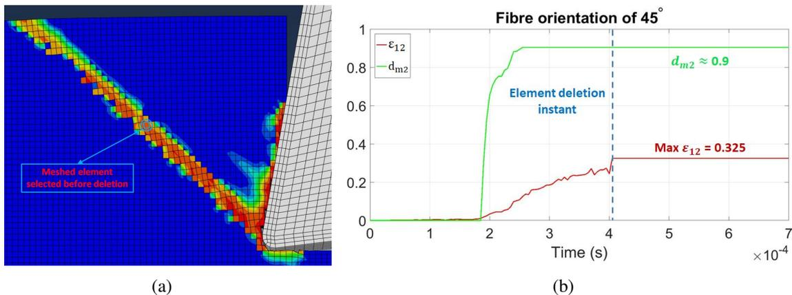
**Fig. 9.** Representation of a representative meshed element deleted to simulate the chip of laminates with a fibre orientation of 45°: (a) Meshed element selected before deletion (b) Evolution of  $d_{m2}$  and  $\epsilon_{12}$  during the simulation time.
