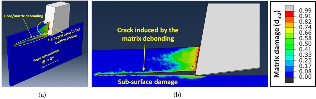
**Fig. 4.** Representation of the FE model simulated with a fibre orientation of  $0^\circ$ : (a) 3D perspective view (b) Front view
