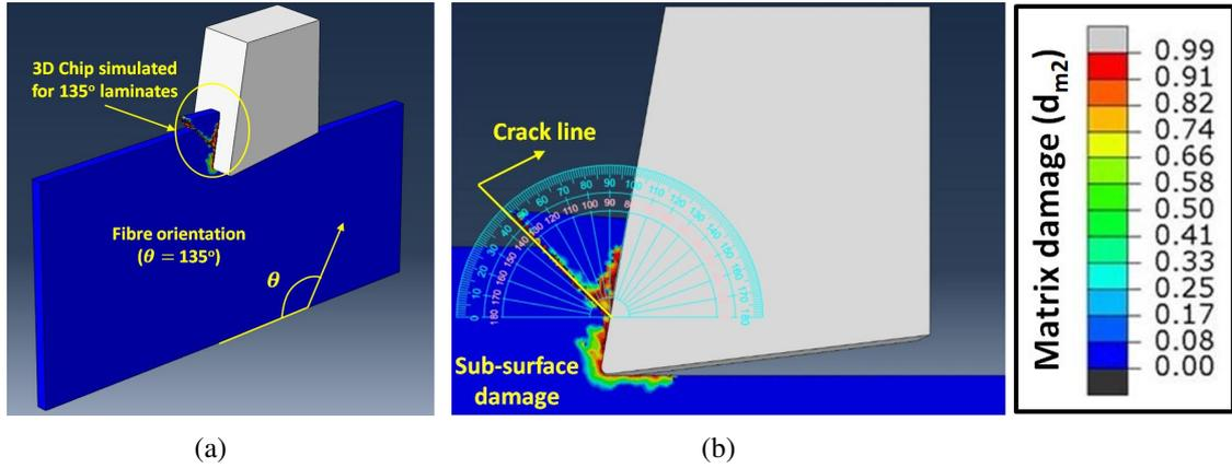
**Fig. 12.** Representation of the FE model simulated with a fibre orientation of 135°: (a) 3D perspective view (b) Front view
