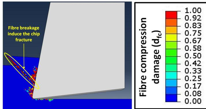
**Fig. 13.** Illustration of the fibre compression damage previous to the chip release in laminates with a fibre orientation of 135°.
