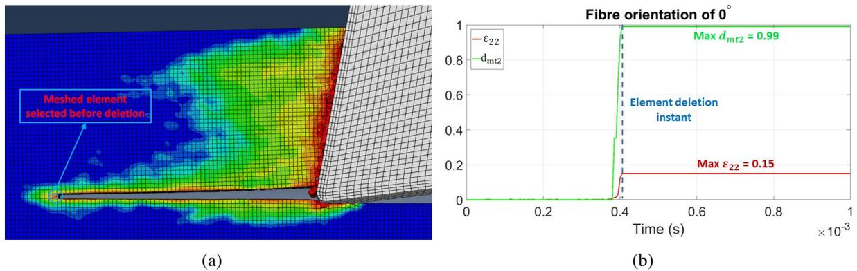
**Fig. 5.** Representation of a representative meshed element deleted to simulate the chip of a laminate with a fibre orientation of  $0^\circ$ : (a) Meshed element selected before deletion (b) Evolution of  $d_{m2}$  and  $\varepsilon_{22}$  during the simulation time.
