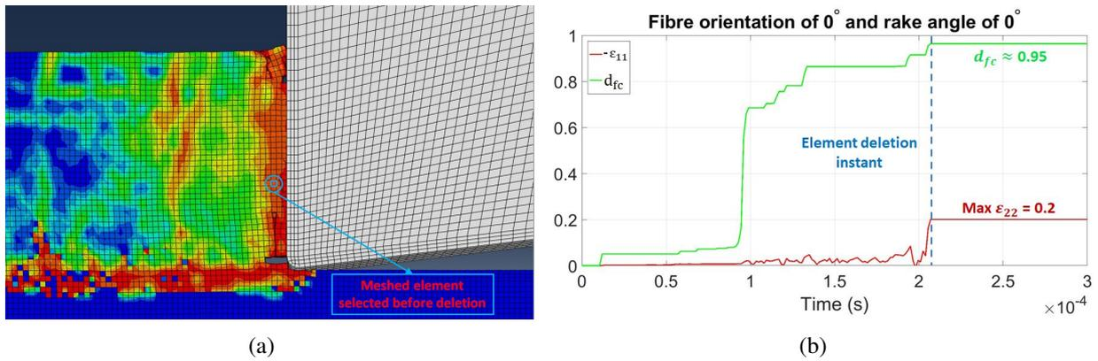
**Fig. 7.** Representation of a representative meshed element deleted to simulate the chip of a laminate with a fibre orientation of  $0^\circ$  and a rake angle of  $0^\circ$ : (a) Meshed element selected before deletion (b) Evolution of  $d_{fc}$  and  $\varepsilon_{11}$  during the simulation time.
