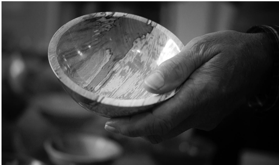
Figure 11.1. A turned bowl showing fungal spalling.
