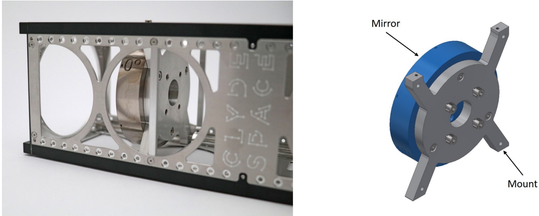
Figure 3. An example of how the mirror from the previous CubeSat study has been integrated within a 3 U CubeSat chassis using a mount - by implementing part consolidation, the mirror and mount could be a single component. Image credit: NSTP3-PF2-008 Team.
