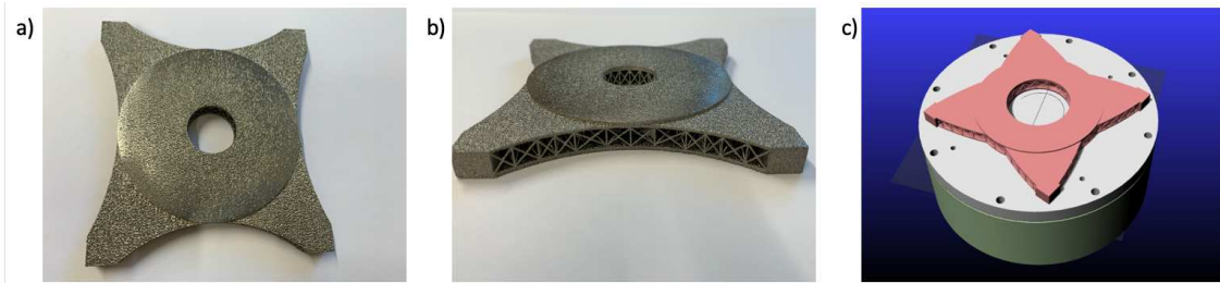
Figure 8. The first design iteration mirror. a) and b) show a prototype built in Ti-6Al-4V using EBM on an Arcam Q20+. c) shows a CAD representation of the design upon a single point diamond turning spindle.
