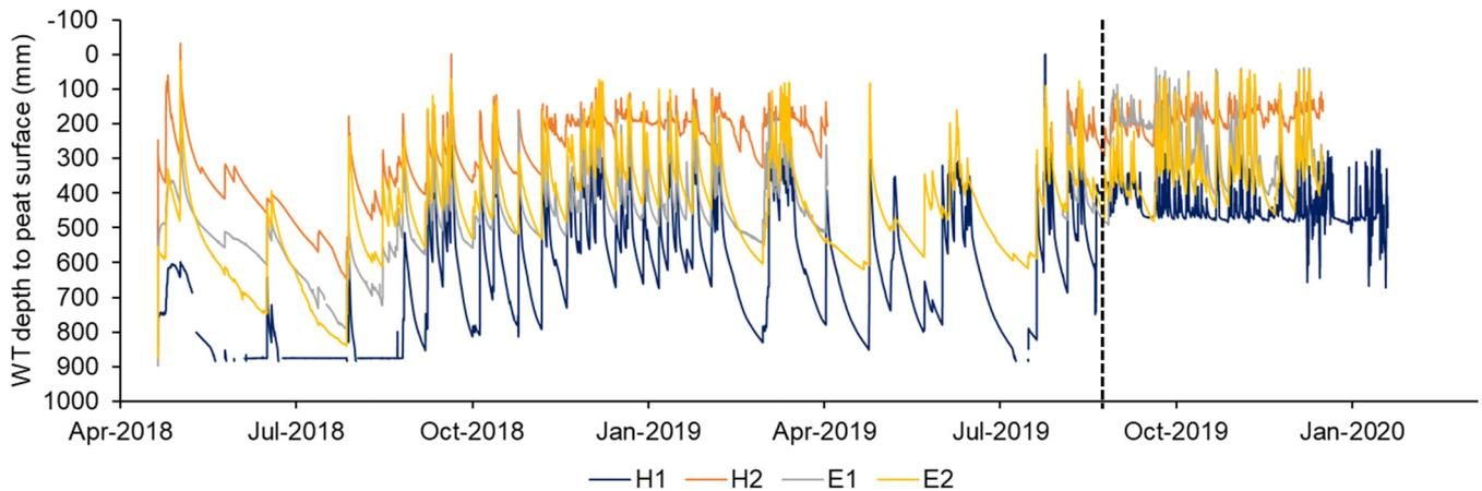
**FIGURE 6** Timeseries of water-table depth at automated dipwell stations for pipes H1, H2, E1 and E2. Vertical dotted line indicated time of blocking pipe outlets
