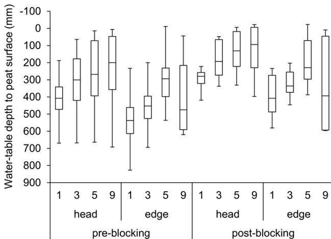
**FIGURE 7** Boxplot of water-table distribution at head and edge locations, across intervention period (pre and post), at 1, 3, 5 and 9 m from the pipe outlet
