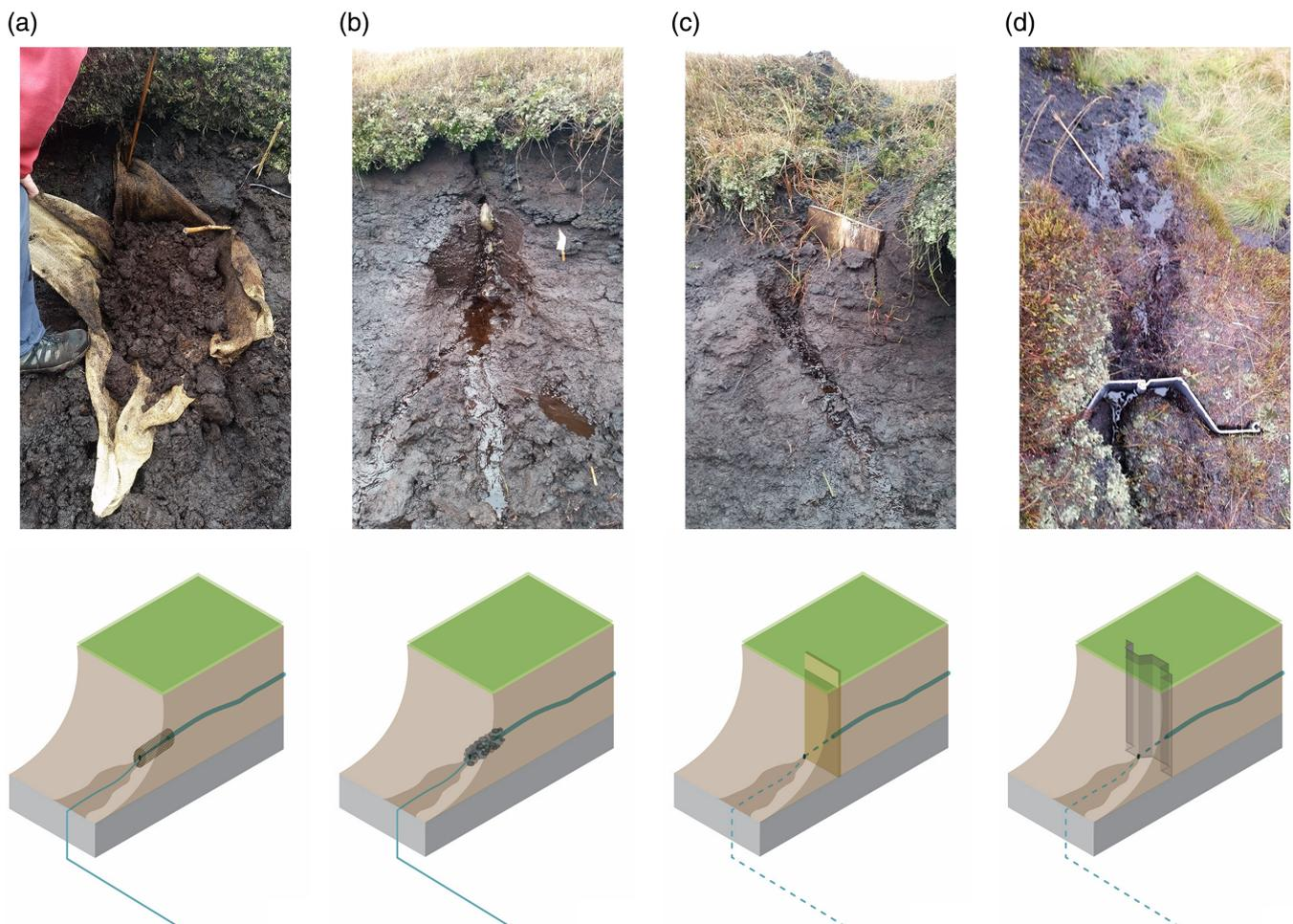
**FIGURE 2** Schematic showing the design and in-field application of plug-like structures and vertical screens to block pipe outlets: (a) jute bag filled with peat, (b) mixture of peat and stones, (c) wooden plank, and (d) plastic pilling. Illustrations produced by P.T.J Lewis
