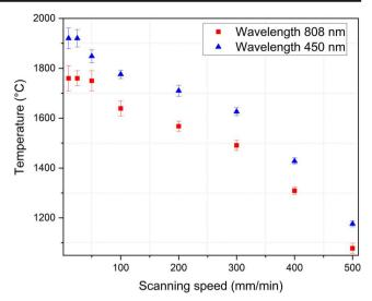
Fig. 8 The maximum temperature measured during laser processing at various scanning speeds for 808-nm and 450-nm wavelengths
