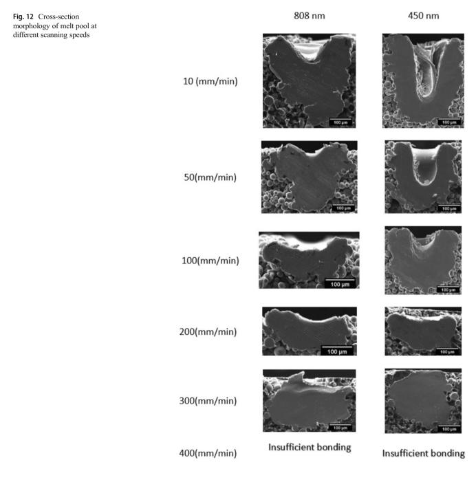
208.2  $\mu$ m when the 450-nm laser was used, compared to 182.8  $\mu$ m for the 808-nm laser. The width of tracks processed using the 450-nm laser remained above 200  $\mu$ m for speeds below 200 mm/min, whereas for 808 nm, the track width narrowed below 200  $\mu$ m at speeds above 50 mm/min.
