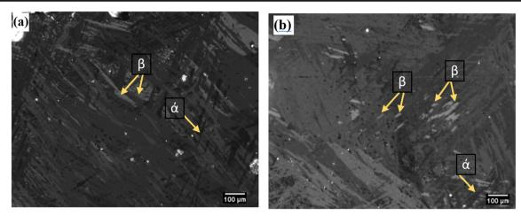
Fig. 20 Ti6Al4V microstructure. a 808 nm. b 450 nm
