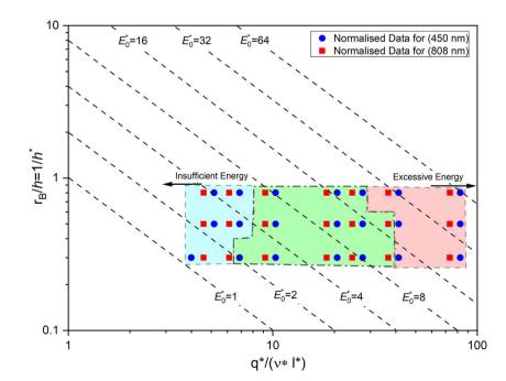
**Fig. 14** Normalised diagram showing the location of the experimental parameters and the visible region for given laser power
