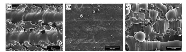
Fig. 16 The effect of hatch distance on the top surface of the specimens.  $\mathbf{a} H_d 200 \ \mu\text{m}$  increase the separation between the tracks.  $\mathbf{b} H_d = 157 \ \mu\text{m}$  is the optimal value to provide better joint and re-melting between tracks.  $\mathbf{c} H_d 100 \ \mu\text{m}$  reduces the processing efficiency and excessive energy
