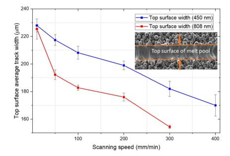
Fig. 11 Effect of scanning speed on melt pool width
