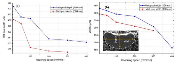
Fig. 13 Variation of melt pool (a) depth and (b) width with scan speed for 450- and 808-nm lasers
