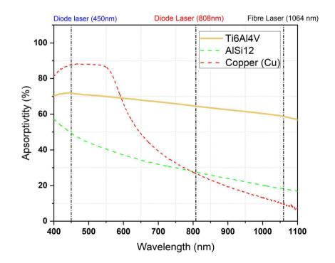
**Fig. 7** The optical absorption of Ti6Al4V, AlSi12 and Cu within the wavelength range of 400 to 1100 nm
