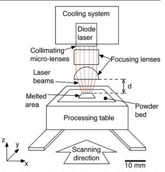
Fig. 1 Diode area melting developed by Zavala et al. [14], individually controllable emitters within moving diode laser bar over powder
