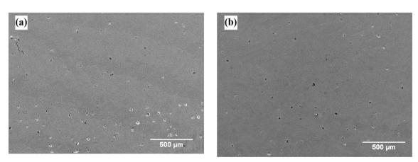
Fig. 18 Top surface porosity of specimen fabricated using (a) 808 nm and (b) 450 nm
