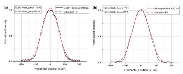
Fig. 4 Beam profiles and Gaussian fit of (a) 808-nm laser module and (b) 450-nm laser module
