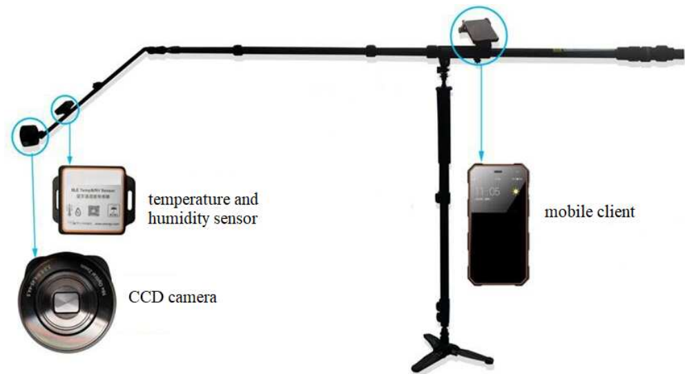
Figure 3. Wild pest image acquisition and pest monitoring equipment.
