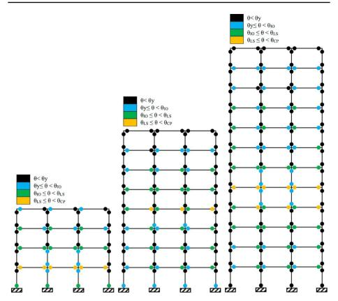
Fig. 13 Distribution of the flexural plastic hinges along the height of original frames under the DBE hazard level  $(R_s)$
