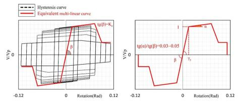
Fig. 7 A sample of the extracted hysteretic response curves for the vertical links and its idealized multilinear equivalent
