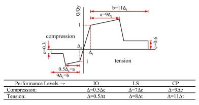
Fig. 9 Load-displacement curve adopted for the modelling of the brace elements in tension and compression and their acceptance criteria based on ASCE/SEI41-17
