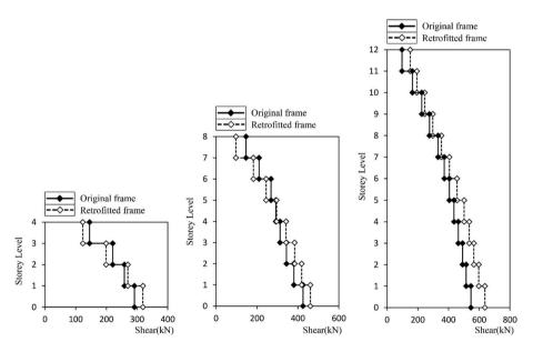
Fig. 12 Mean value of the maximum storey shear forces under the DBE hazard level before and after the retrofitting
