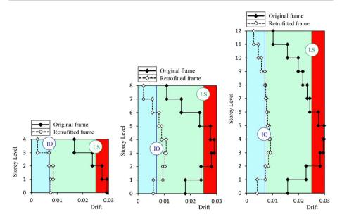
Fig. 11 Mean value of the maximum drifts under the DBE hazard level before and after the retrofitting
