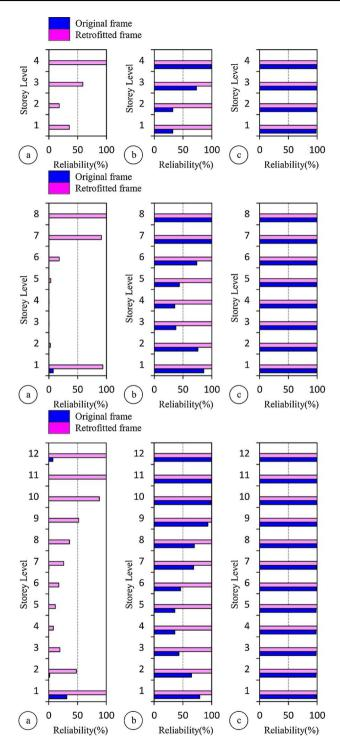
Fig. 16 Reliability of MRFs for not exceeding the performance levels of a IO, b LS, c CP
