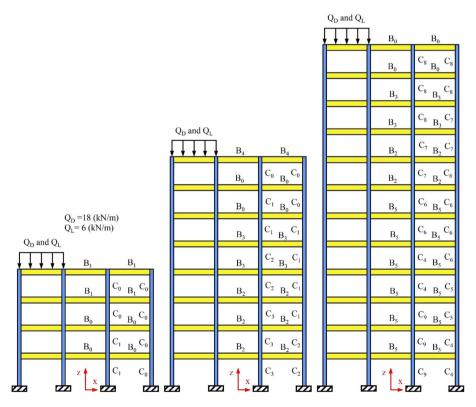
Fig. 2 Geometric characteristics and gravity loading of the moment-resisting frames to be retrofitted
