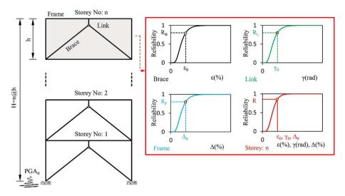
Fig. 24 Process of extracting reliability curves for each storey (schematic)
