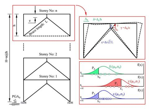
**Fig. 19** Schematic representation of calculating the reliability of different groups of members for a hypothetical performance level  $(x_0, x_1, x_2)$  under a certain hazard level  $(PGA_0)$
