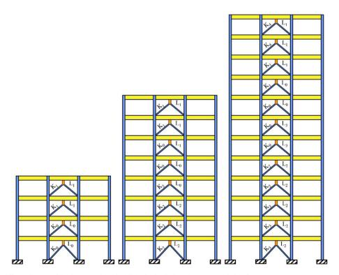
Fig. 6 Layout of the braces and vertical links in the designed moment-resisting frames
