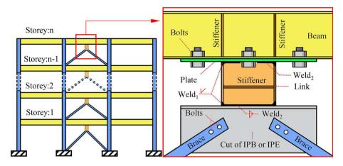
Fig. 1 Eccentric braced frame equipped with vertical link beam and schematic details of the link connection
