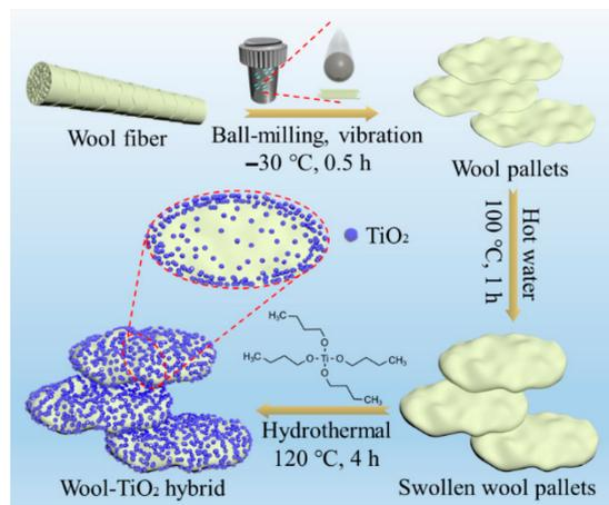
**Figure 8.** Schematic illustration for the fabrication of the WT hybrid composite powders.
