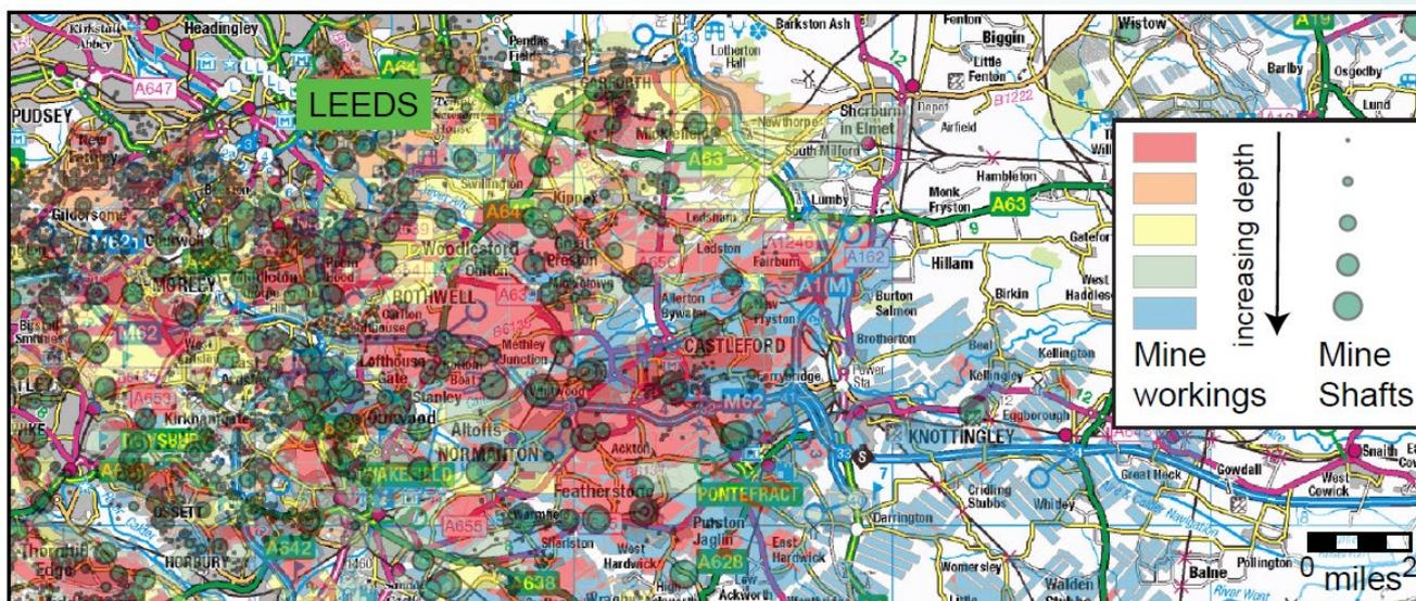
**Map of Leeds showing legacy mine workings (Coal Authority Data). Most of the area is underlain by mine workings with associated shafts at various depth illustrating the potential to use these for heat and energy storage as well as heat generation in cities with mining history.**
