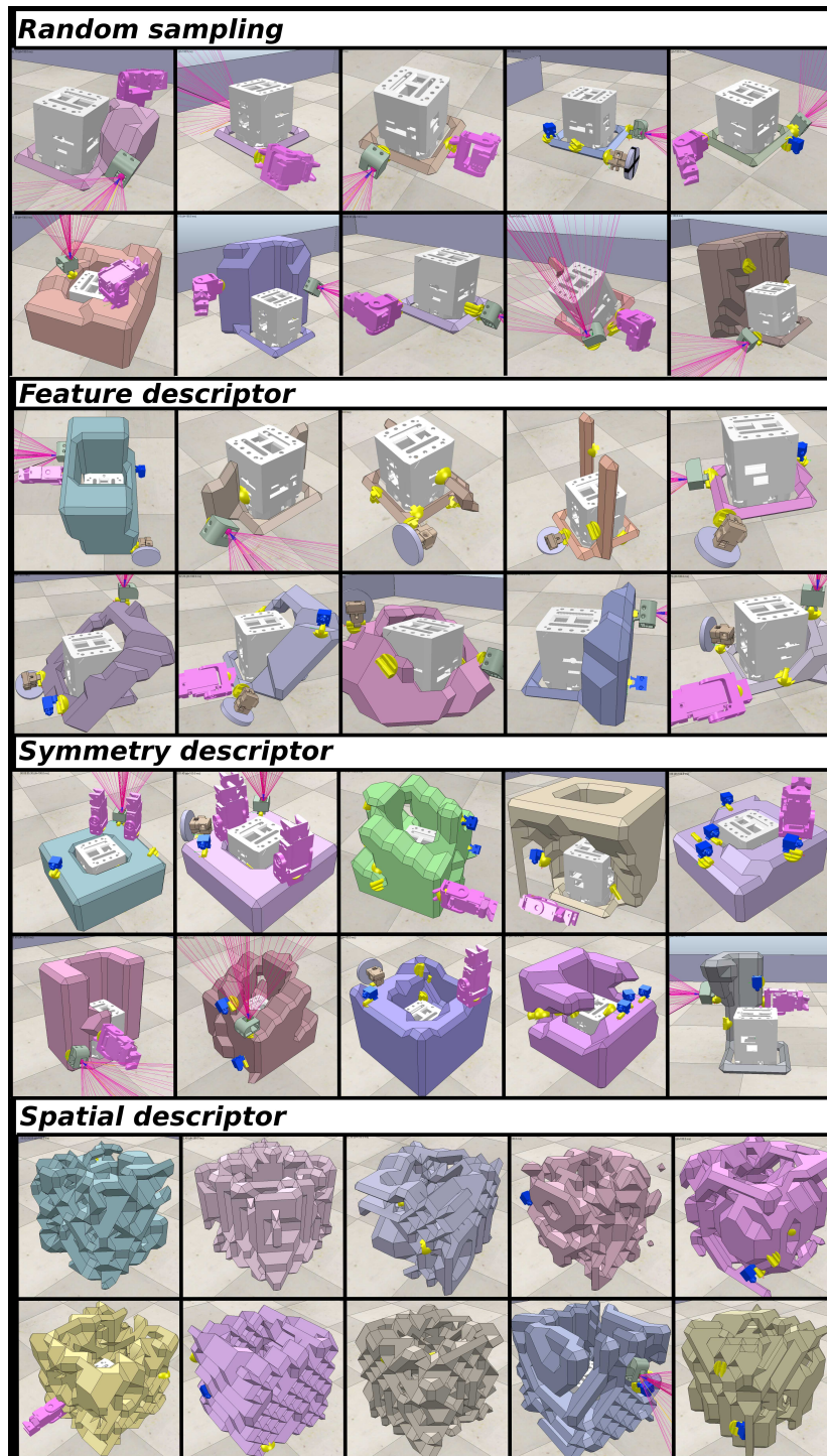
Figure 5. Body plans generated with random sampling and evolved with each descriptor (feature, symmetry and spatial). The descriptors define the final features in the robots. The feature descriptor generates the robots with highest number of organs and low skeleton complexity. The spatial descriptor generates the robots with the lowest number of organs but with high skeleton complexity. The symmetry descriptor sits in the middle of the previous descriptors.
