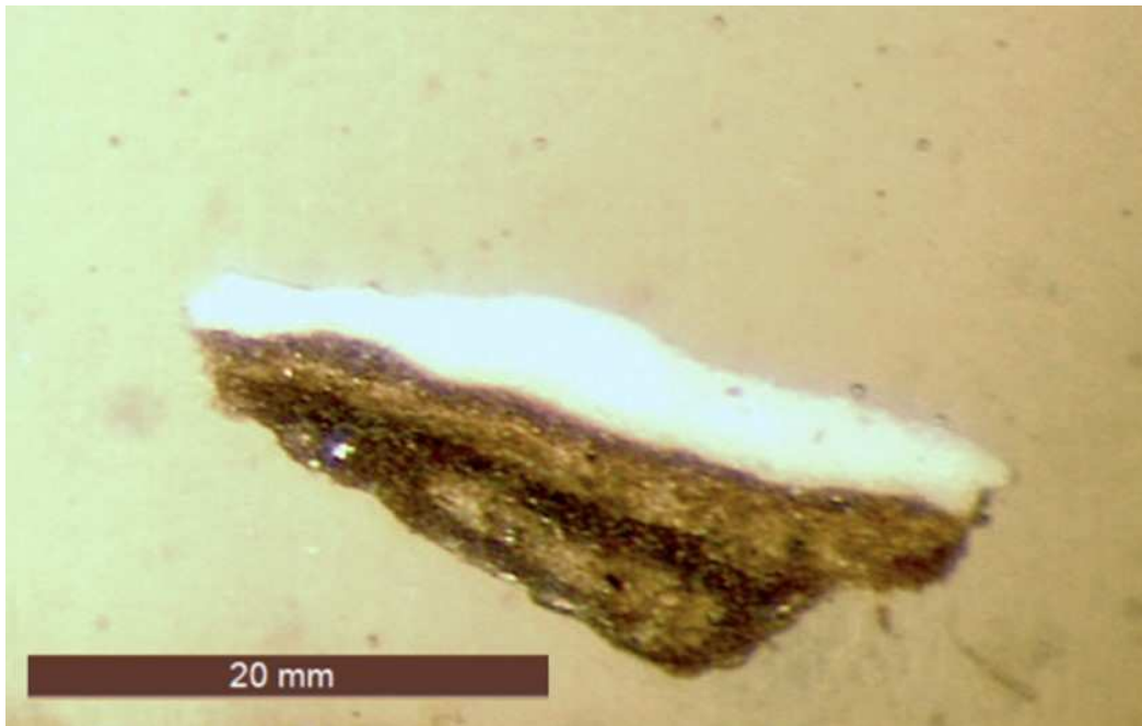
Figure 11. Cross-section taken from female deity's cheek, photographed under LEICA Microscope, light grey (sample taken after varnish removal and before a contemporary varnish application). Photograph by the author, 2020.
