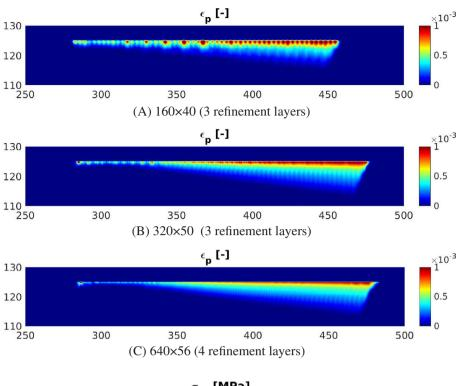
**FIGURE 13** Plastic strain after t = 1.2 s around the right fracture tip using a standard continuum with  $\eta \sigma_0 = 10^5$  Pa·s. (A)  $160 \times 40$  (three refinement layers); (B)  $320 \times 50$  (three refinement layers); (C)  $640 \times 56$  (four refinement layers) [Color figure can be viewed at wileyonlinelibrary.com]
