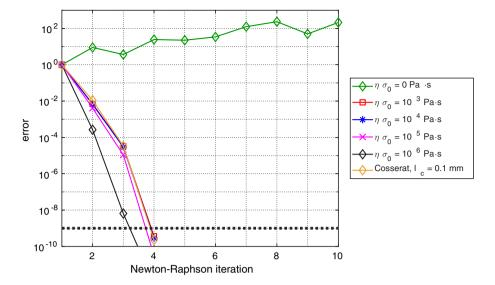
**FIGURE 5** Convergence behavior for a standard continuum with and without viscoplasticity, and using a Cosserat continuum without viscoplasticity for  $t_t = 0.2$  MPa,  $\Delta t = 0.1$  ms [Color figure can be viewed at wileyonlinelibrary.com]
