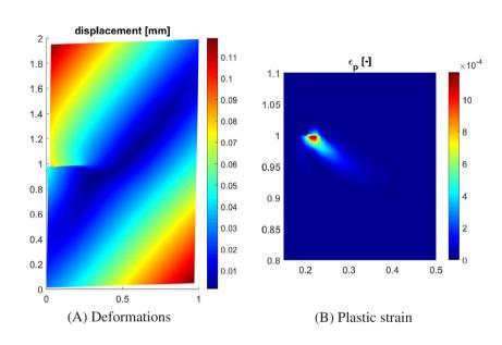
**FIGURE 3** Deformations and plastic strain at t = 1.02 s for  $t_t = 0.4$  MPa [Color figure can be viewed at wileyonlinelibrary.com]
