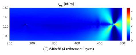
**FIGURE 14** Shear stress at t = 1.2 s around the right fracture using a Cosserat continuum. (A)  $160 \times 40$  (three refinement layers); (B)  $320 \times 50$  (three refinement layers); (C)  $640 \times 56$  (four refinement layers) [Color figure can be viewed at wileyonlinelibrary.com]
