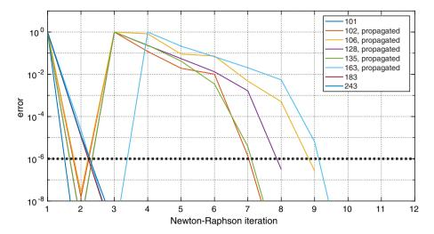
**FIGURE 10** Convergence during selected time steps without Cosserat continuum ( $\eta \sigma_0 = 10^5 \text{ Pa} \cdot \text{s}$ ) using the  $160 \times 40 \text{ mesh with } \Delta t = 1.0 \text{ ms [Color figure can be viewed at wileyonlinelibrary.com]}$
