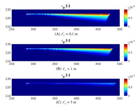
**FIGURE 17** Plastic strain after t = 1.2 s around the right fracture tip using a Cosserat continuum with the  $320 \times 50$  mesh. (A) $\ell_c = 0.1$  m (B) $\ell_c = 1$  m (C) $\ell_c = 5$  m [Color figure can be viewed at wileyonlinelibrary.com]
