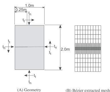
**FIGURE 2** Geometry and mesh used for the case without fracture propagation. (A) Geometry; (B) Bézier extracted mesh
