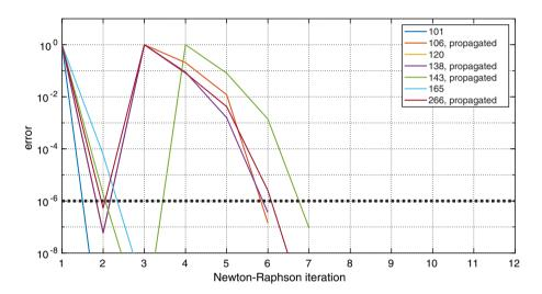
**FIGURE 11** Convergence during selected time-steps using a Cosserat continuum ( $\ell_c = 10 \text{ mm}$ ) using the  $160 \times 40 \text{ mesh with } \Delta t = 1.0 \text{ ms}$  [Color figure can be viewed at wileyonlinelibrary.com]
