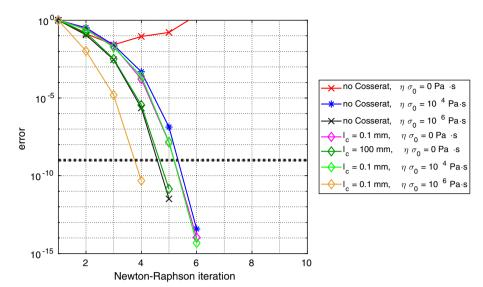
**FIGURE 6** Convergence behavior for a standard continuum, and for a Cosserat continuum for  $t_t = 0.4$  MPa,  $\Delta t = 1$  ms [Color figure can be viewed at wileyonlinelibrary.com]
