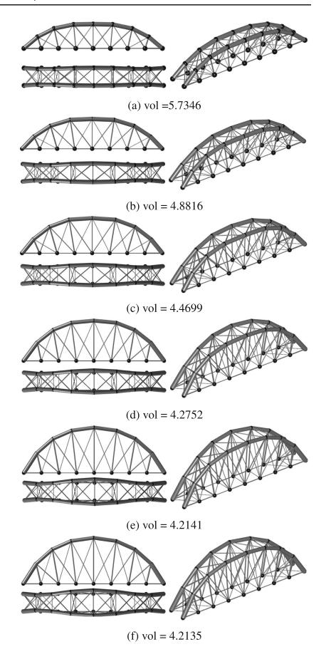
Example 6 Here, we start with the solution of the bridge problem shown in Fig. 2e, where the top four corner nodes in the design space of Fig. 2a are no longer present. The entire process is demonstrated in Table 6 and Fig. 7. No nodes are melted or merged in this case. The final design
