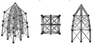
(d) vol = 0.1230, moving joints, with stability constraints
