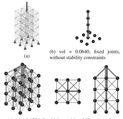
(c) vol = 0.1536, fixed joints, with stability constraints
