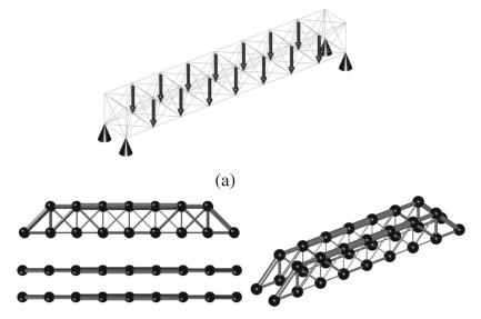
(b) vol = 10.3253, fixed joints, without stability constraints
