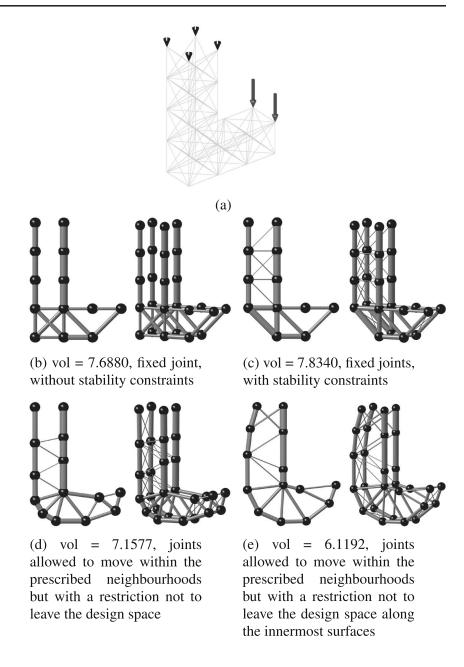
which is obtained by solving the problem with stability constraints. Next, we solve the problem for moving joints. First, the joints are allowed to move in a neighborhood of radius r=0.4 but are restricted to remain within the
