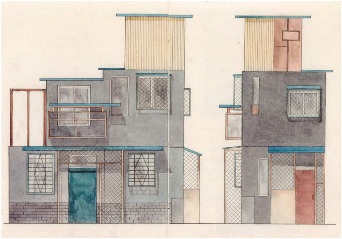
Figure 5 Drawing of a three-floor concrete house with self-build elements in light-weight, affordable industrial materials
