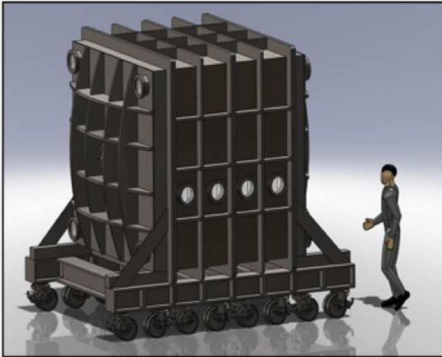
FIG. 31. Design for a first stage 8 \text{ m}^3 steel vessel (courtesy of D. Warner, Colorado State University).
