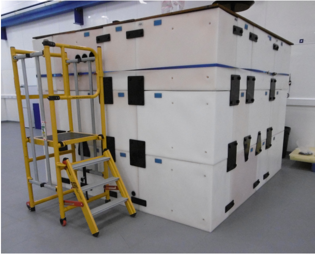
FIG. 32. DRIFT-IIId interlocking acrylic block shielding surrounding the detector and containing water, located at Boulby underground laboratory.
