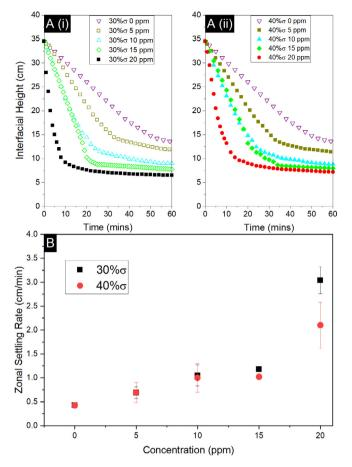
**Fig. 6.** (A) Interface height versus time for flocculated 2.5 vol.%  $Mg(OH)_2$  with varying concentrations of (i) 30%  $\sigma$  and (ii) 40%  $\sigma$  polymer, prepared in a reactor agitated at 300 rpm for 1000 s. (B) Linear zonal settling rate versus polymer concentrations for the same systems.
