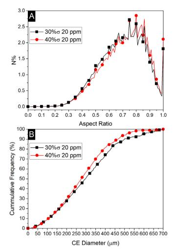
**Fig. 3.** (A) Aspect ratio distribution and (B) cumulative frequency distribution, for optical image analysis of 2.5 vol.% Mg(OH)<sub>2</sub> suspensions agitated for 1000 s at 300 rpm with  $30\%\sigma$  and  $40\%\sigma$  polymers dosed at 20 ppm.
