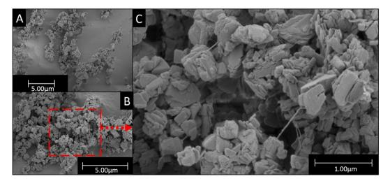
Fig. 5. Cryo-SEM images of 2.5 vol.% Mg(OH)<sub>2</sub> suspensions mixed with 20 ppm 40%σ polymer. (A) 19982x magnification, (B) 35000x magnification and (C) 99959x magnification.
