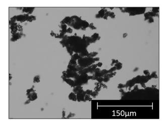
Fig. 4. Example optical microscope image of  $Mg(OH)_2$  suspensions mixed with 20 ppm 30%  $\sigma$  polymer.
