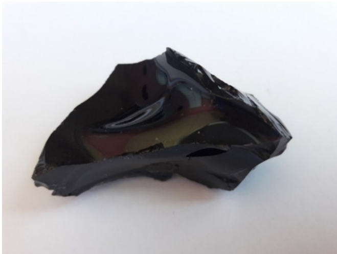
Fig. 3. Waste glass sample from the SHIVA trial.
