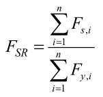
$F_{SR}$ : slip Load Ratio  $F_{s,i}$ : slip load of the  $i^{th}$  storey  $F_{y,i}$ : storey shear strength
