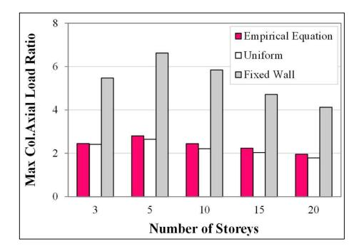
Axial load in the columns is significantly reduced
