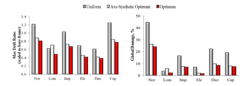
Average of optimum slip load patterns for a set of a spectrum compatible earthquakes can be used for practical design purposes
