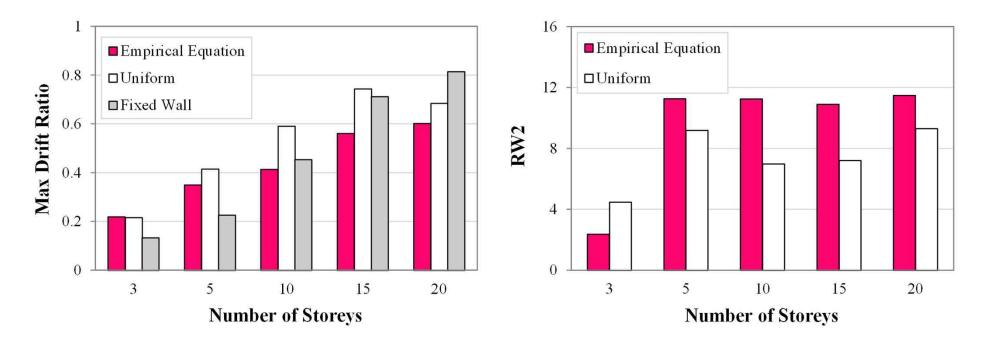
By increasing the energy dissipation, maximum inter-storey drift is reduced compared to conventional design method
