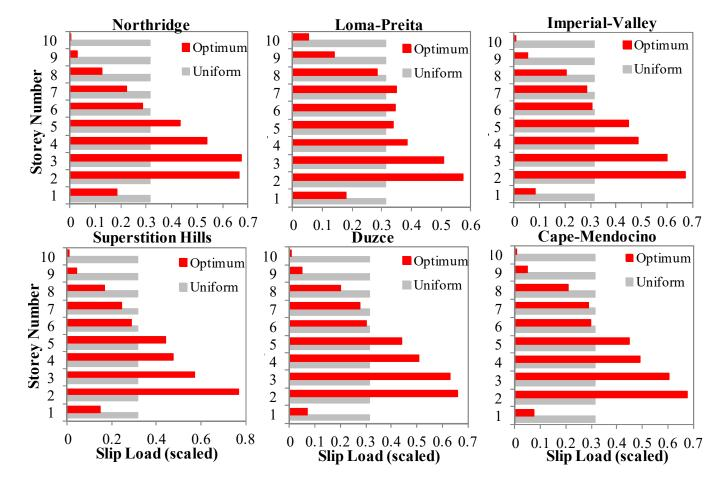
Comparison between optimum and uniform distribution of slip loads (scaled to the average storey shear strength) for 10-storey frames under six natural earthquakes
