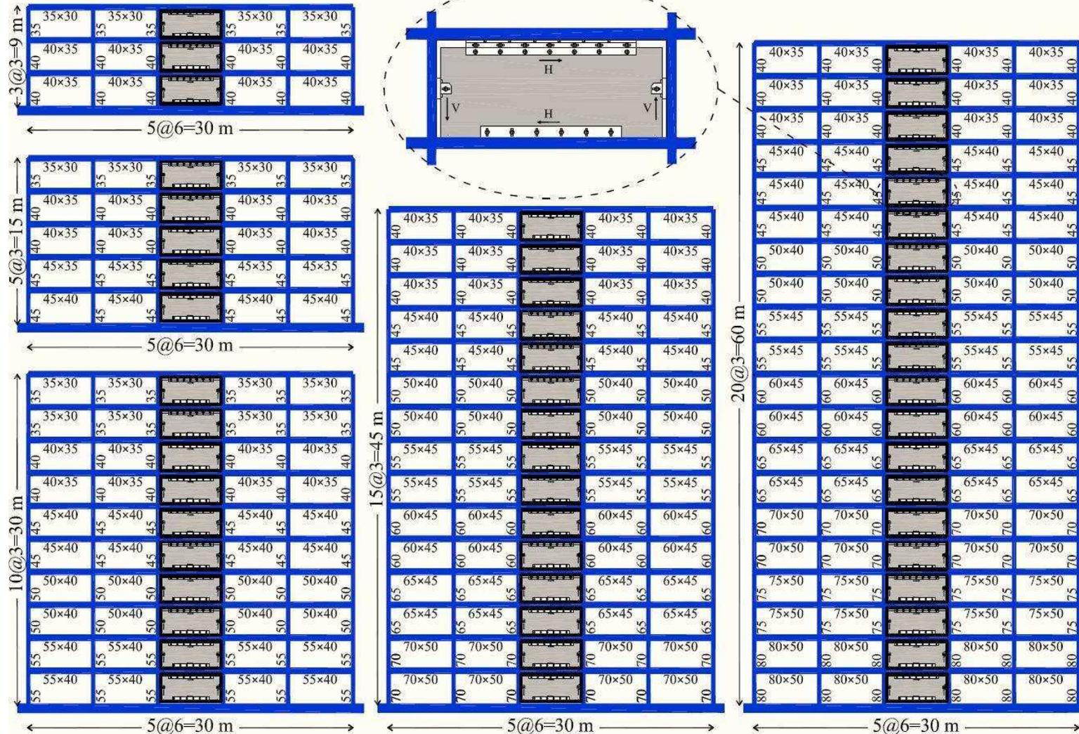
Geometry of the reference RC frames equipped with friction wall dampers
