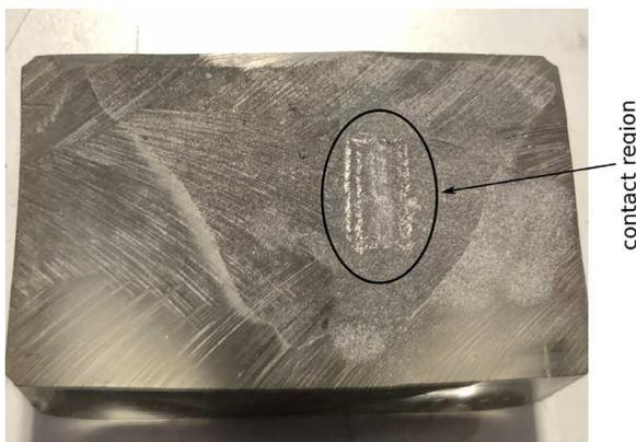
(b) flat specimen after friction testing, including wear scar
