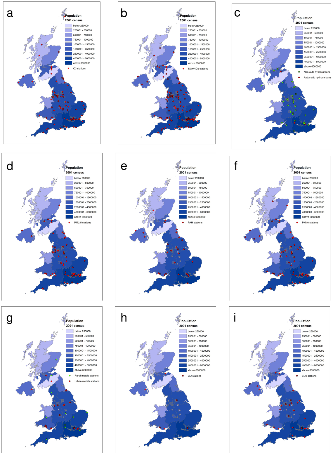
Figure 3: Location of Defra measurement sites (early 2013) and their relation to UK population for: (a) ozone; (b) \text{NO}_x/\text{NO}_2 ; (c) hydrocarbons; (d) \text{PM}_{2.5} ; (e) PAHs; (f) \text{PM}_{10} ; (g) rural and urban metals; (h) CO; and (i) \text{SO}_2 .
