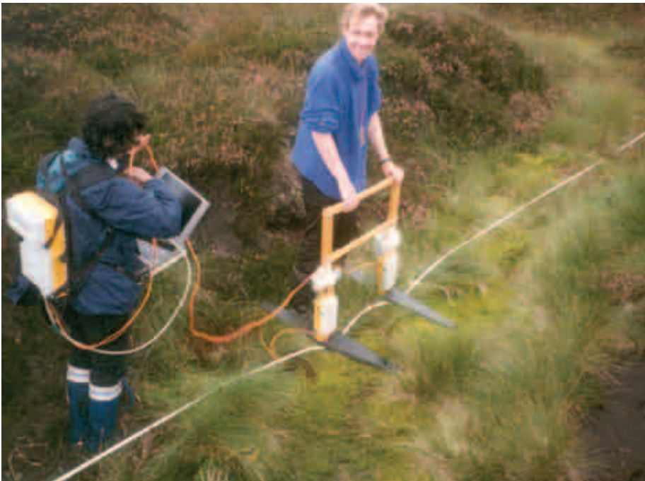
Figure 2. Mapping soil pipes using ground-penetrating radar. The instrument is transported or wheeled across the surface and can detect soil pipes that are several meters below the surface.
