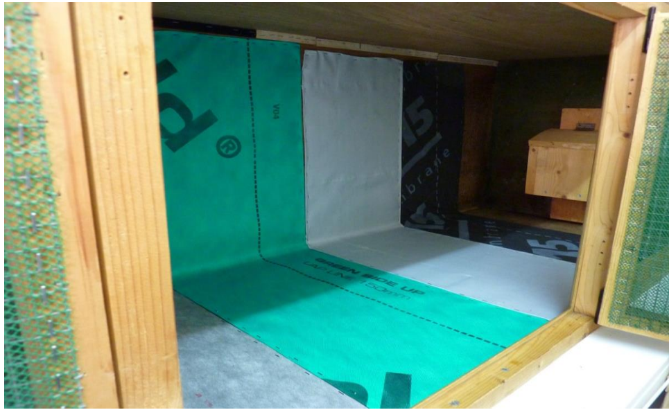
Figure 10. Photograph showing the four test specimens fitted inside the pipistrelle aviary
