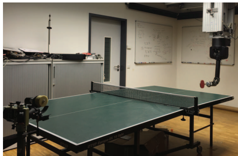
Fig. 1: The 7-DoF robot table tennis setup.
