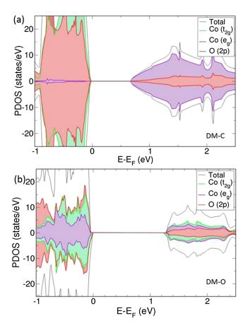
FIG. 4. PDOS for (a) cubic and (b) orthorhombic diamagnetic SmCoO<sub>3</sub>.
