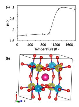
FIG. 10. (a) Cobalt magnetic moment in the cubic CAFM magnetic structure as a function of temperature (K). (b) Structure of the pseudo-cubic CAFM structure  $SmCoO_3$  at 1273 K. Please note that the temperature is related to the supercell volume.
