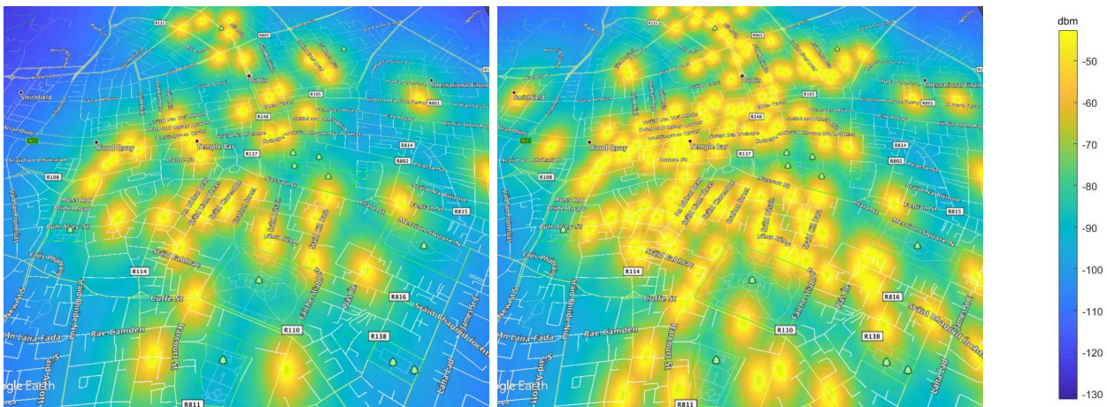
Fig. 3: RSS in Dublin city centre from small cells deployed in all hotels (right) and chain hotels only (left). The list and locations of all hotels in the area was obtained using google place API.
