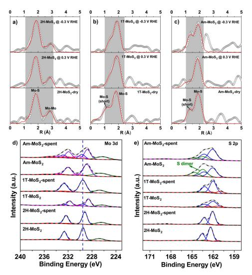
**Figure 3.** a-c) Mo K-edge Fourier transform EXAFS ( $k^2$ -weighted) of 2H- (a), 1T- (b), and Am- (c) MoS<sub>2</sub> under operando electrochemical conditions. Gray region represents R-range for fitting. d, e) X-ray photoemission spectra of Mo3d (d) and S2p (e) before and after (spent) operando XAS measurements.
