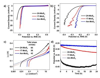
**Figure 1.** a, b) Cyclic voltammetry (CV; a) and linear sweep voltammetry (LSV; b) curves of 2H-, 1T-, and Am-MoS<sub>2</sub> films corrected by uncompensated resistance with scan rates of 50 mV s<sup>-1</sup> for CV and 5 mV s<sup>-1</sup> for LSV. c) Tafel slopes obtained from LSV curves in (b). d) Chronopotentiometric responses (*V*-*t*) recorded at a constant current density of 3 mA cm<sup>-2</sup>. Electrolyte:  $0.1 \text{ M H}_2\text{SO}_4$ .
