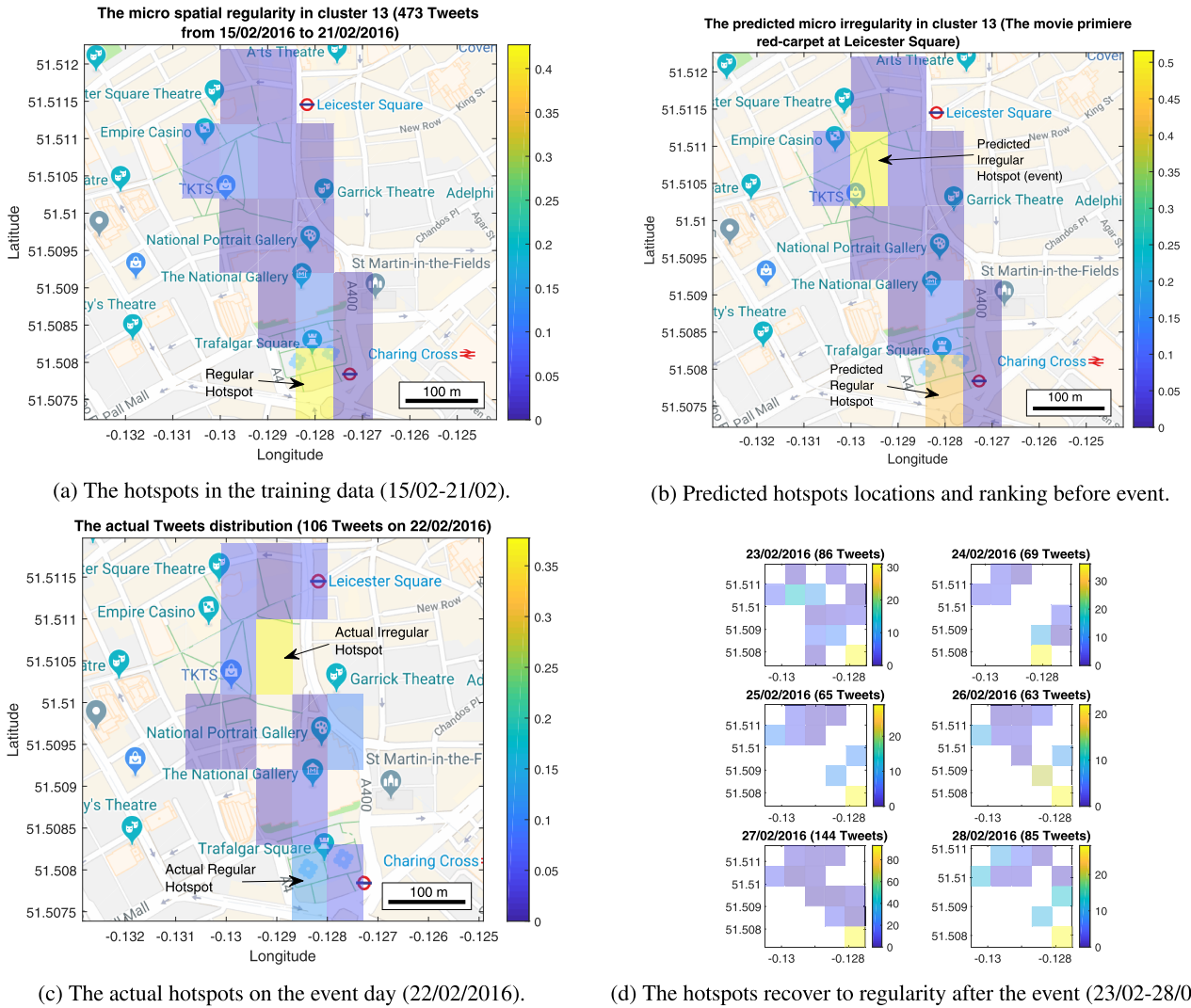
FIGURE 7. The actual and predicted traffic patterns before and after the event. We transfer the Tweets distribution in cluster 13 into a histogram that describes the Tweets occurrence in each pixel. The pixel with more Tweets is regarded as a hotspot. The regular hotspot is usually attractive for users. In contrast, the irregular hotspot brings a sudden burst of Tweets and disappears after the event.
