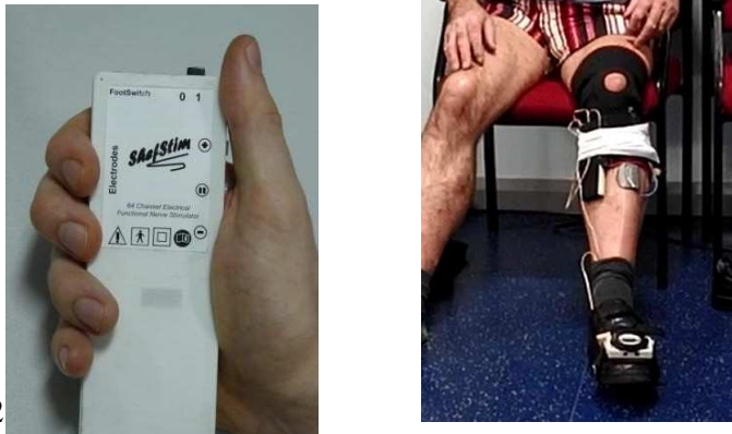
382 383 Figure 5: ShefStim stimulator (left) being used by a subject during setup (right)
