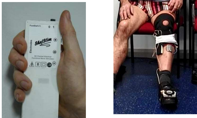
342 Figure 5: ShefStim stimulator (left) being used by a subject during setup (right)
