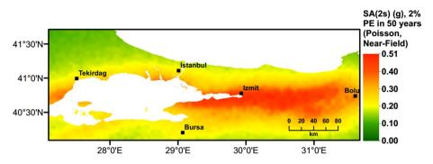
Fig. 23 Seismic hazard map of Marmara region for SA (g) T=2.0 s considering 2% probability of exceedance in 50 years employing the Poisson model including near-field directivity effects
