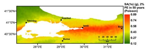
Fig. 22 Seismic hazard map of Marmara region for SA (g) T=1.0 s considering 2% probability of exceedance in 50 years (the Poisson model)
