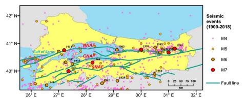
Fig. 9 Faults system in Marmara region with epicentral location of major earthquakes occurred in twentieth century (Faults data is taken from https://www.efehr.org)
