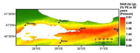
Fig. 20 Seismic hazard map of Marmara region for SA (g) T=0.2 s considering 2% probability of exceedance in 50 years (the Poisson model)
