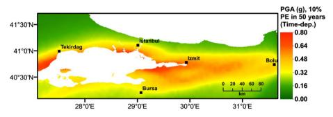
**Fig. 16** Seismic hazard map of Marmara region for PGA (g) considering 10% probability of exceedance in 50 years (Time-dependent model)
