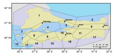
Fig.11 Background source model used in the PSHA presented in this study. Zone numbers and corresponding parameters are listed in Table 3
