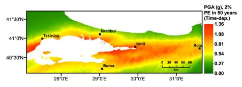
Fig. 18 Seismic hazard map of Marmara region for PGA (g) considering 2% probability of exceedance in 50 years (Time-dependent model)
