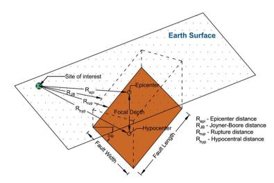
Fig. 3 Fault geometry and projection on to the surface with distance metrics used in GMPEs
