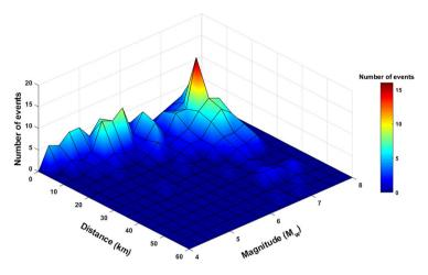
**Fig. 26** Design earthquakes in terms of distance and magnitude for a design PGA =  $0.35 \text{ g} (\pm 0.01 \text{ g})$  for a location in Istanbul, with POE of 10% in 50 years and calculated using a Poisson model
