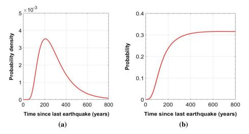
Fig. 6 a PDF and b conditional probability for BPT distribution with a mean return period of 300 years and  $\alpha = 0.5$
