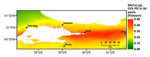
Fig. 21 Seismic hazard map of Marmara region for SA (g) T = 1.0 s considering 10% probability of exceedance in 50 years (the Poisson model)
