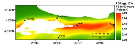
**Fig. 15** Seismic hazard map of Marmara region for PGA (g) considering 10% probability of exceedance in 50 years (the Poisson model)
