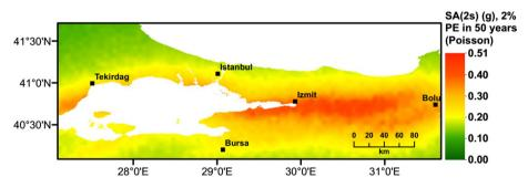
Fig. 24 Seismic hazard map of Marmara region for SA (g) T=2.0 s considering 2% probability of exceedance in 50 years (the Poisson model)
