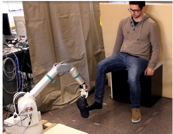
Fig. 1. Assisted-dressing scenario with a WAM robot: use case of putting on a shoe.
