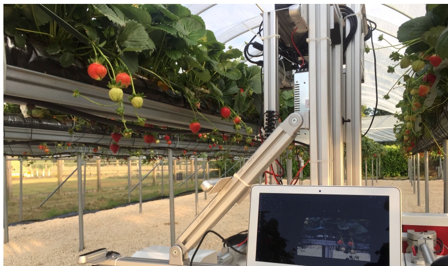
Figure 5. The image acquisition rig inside the strawberry polytunnels.
