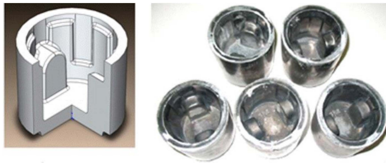
Figure 15. Piston three-dimensional (3D) model, pistons thixoformed in the AJ125 alloy [49] (Courtesy of Prof. Boris Ivanovich Semenov).
