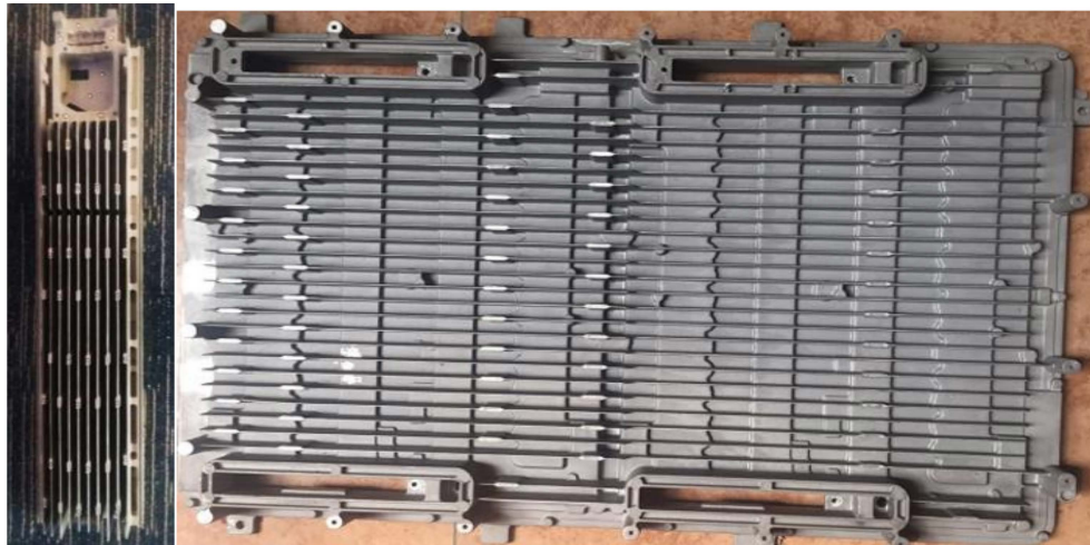
Figure 10. Large components incorporating thin parts. Left: 4G antenna case shell, size: 793 \times 166 \times 86 mm, addendum thickness: 1 mm. Right: communication base station cooling shell, size: 733 \times 470 \times 46 mm, addendum thickness: 1.1 mm [33] (Courtesy of Mingfan Qi, School of Materials Science and Engineering, University of Science and Technology Beijing).
