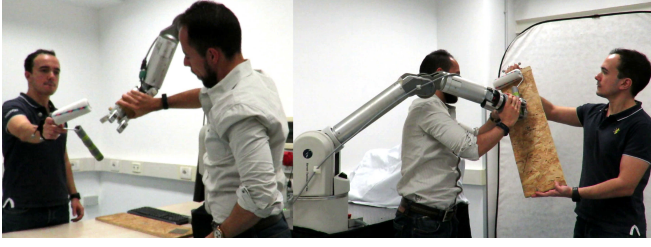
Fig. 8: Two persons demonstrate the painting task to the robot. Left: The robot is shown how to receive the paint roller. Right: One person drives the robot to demonstrate the painting strokes, while the other holds the board.
