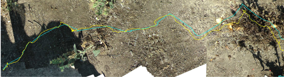
Figure 4: Trajectory projection example (clutter scenario from Table 1; see also Figure 5 (A)). The cyan line represents the sparse trajectory based on the key-frames only and the yellow line represents the dense track from all frames.
