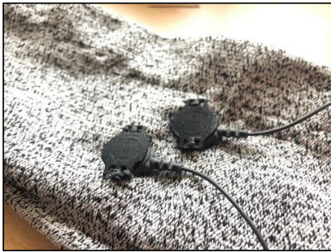
FIGURE 10 - THE SLEEVE INSIDE-OUT. THIS SHOWS HOW THE ELECTRODES WERE STITCHED ONTO THE SLEEVE
