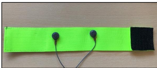
FIGURE 6 - SNAP-ON ELECTRODES SEWED ONTO THE ARMBAND
