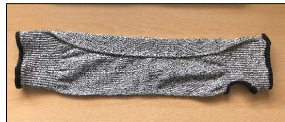
FIGURE 9 - THE SLEEVE TO BE USED AS THE WEARABLE. IT WAS FOLDED AND STITCHED TO MAKE IT TIGHTER ON THE FOREARM AND HENCE ENSURE BETTER ELECTRODE-SKIN CONTACT
