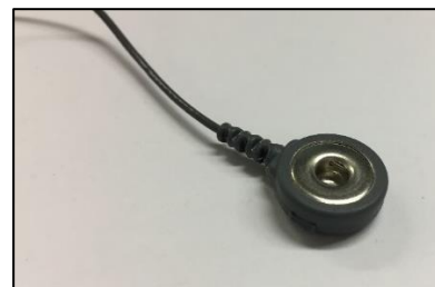
FIGURE 2 - THE STANDARD ELECTRODE CABLE
