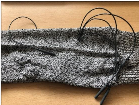
FIGURE 11 - SHOWING HOW THE ELECTRODE CABLES WERE FORCED THROUGH THE WEARABLE TO ATTACH THEM TO THE SHIMMER SENSOR ON THE OUTSIDE
