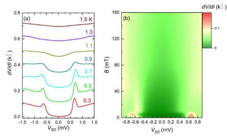
Figure 5. The temperature and magnetic field dependence of induced superconductivity in e-beam lithographically fabricated junctions. (a) Induced superconducting gap vs. applied source-drain voltage  $V_{SD}$  at temperatures between 300 mK and 1.5 K. The curves are vertically offset for clarity. (b) Color-coded differential resistance as a function of  $V_{SD}$  and perpendicular magnetic field at T= 300 mK. Please click here to view a larger version of this figure.
