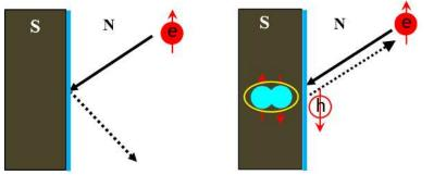
Figure 3. Normal and Andreev Reflections in hybrid superconducting-semiconducting junctions. (a) Specular quasiparticle reflection with no charge transmission through the interface. (b) Andreev reflection whereas the incoming electron is reflected as a hole in the opposite spin sub-band and transfer 2e charge into superconducting electrode. Please click here to view a larger version of this figure.
