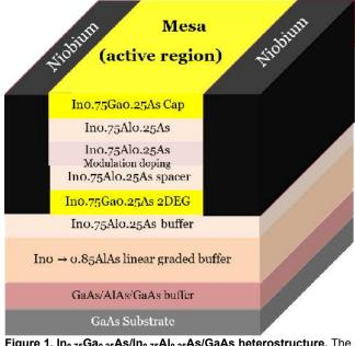
**Figure 1.**  $In_{0.75}Ga_{0.25}As/In_{0.75}Ga_{0.25}As/GaAs$  heterostructure. The schematic view of the heterojunction where an  $In_{0.75}Ga_{0.25}As$  quantum well with 30 nm thickness is formed #120 nm below the wafer surface. Nb was used as the superconducting contacts (shown in black) to form a hybrid and ballistic Nb–In<sub>0.75</sub>Ga<sub>0.25</sub>As 2DEG–Nb Josephson junction. Please click here to view a larger version of this figure.
