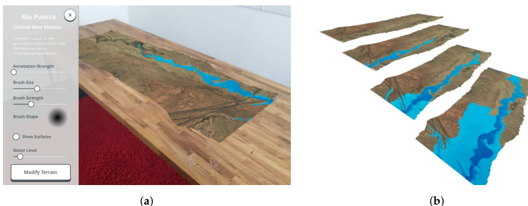
Figure 5. Flood Visualisation (a) A screenshot of the flood visualisation software in use (b) A visualisation of water level progression using our built-in flood simulator. Underlying DEM data from the 2010 Rio Puerco River Study of overbank flood dynamics [22].
