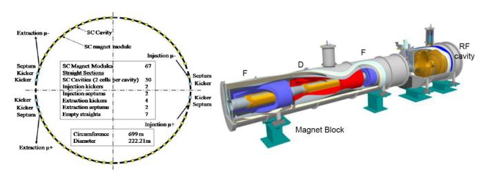
FIG. 12. Left: NS-FFAG layout presented in the IDS-NF IDR [21]. Right: engineering concept for the cryo-modules including three magnets and one cavity.
