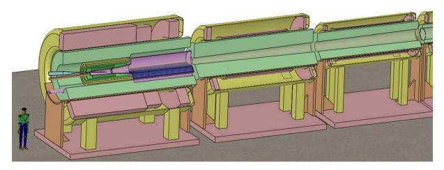
FIG. 5. Schematic of the EURO $\nu$  baseline Neutrino Factory target station using a free flowing mercury jet and capture solenoid.
