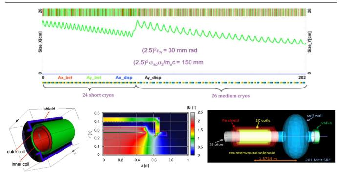
FIG. 9. Top panel: Layout of the muon linac consisting of 24 one cavity modules and 26 two cavity modules to achieve a final energy of 0.9 GeV. The lower left-hand panel shows an electromagnetic model of the superconducting solenoid, the lower center panel shows the field distribution at the end of the solenoid and the lower right-hand panel shows one short cryo-module.
