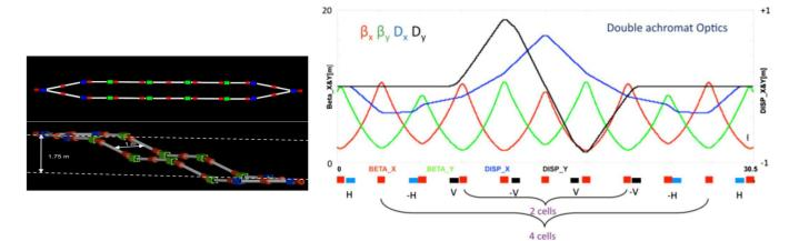
FIG. 10. Left: Layout of the injection chicane from the muon linac into the first RLA in two projections. Right: lattice details of the injection chicane in OptiM.
