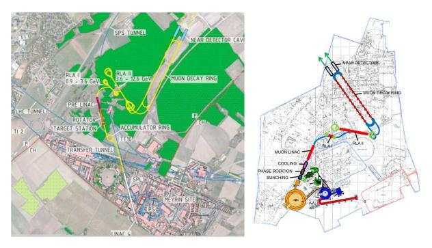
FIG. 14. Layout of the EURO $\nu$  baseline neutrino factory on the two sites considered by EURO $\nu$ . Left: Layout at CERN in which SPL servers accumulator and compressor rings and the muon-accelerator complex is laid out in the North Area. Right: Layout at RAL in which an upgrade of ISIS serves an RCS and the muon-accelerator complex is laid out on the Harwell Campus.
