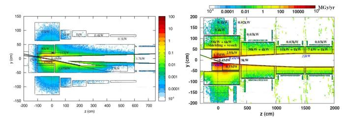
FIG. 4. Simulation of power dissipation due to radiation in the target station region for the Study 2a target design [56] (left panel) and the EURO $\nu$  baseline target station (right panel).
