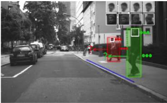
Fig. 1. Pedestrian intention with a vehicle, from its dashcam, in the Daimler dataset [17]. The present study uses a heuristic model to predict the outcomes of interactions from this data – whether the pedestrian will cross in front of the vehicle or yield to it.
